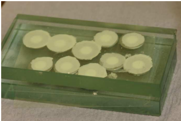
Figure 2: Example of 11mm Diameter Cement Disks Setting
