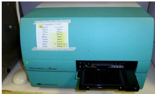
Figure 6: Fluorimeter with Black 96-Well Plate
