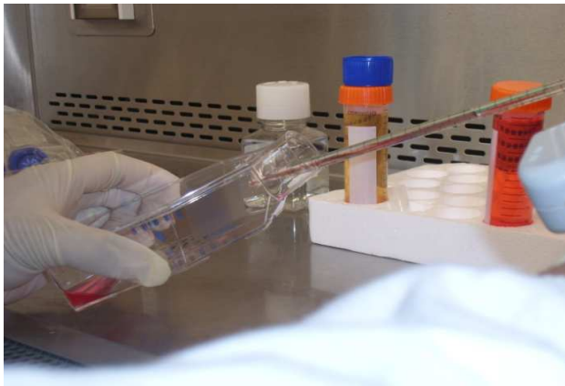
Figure 4: Addition of Medium to 75cm 2 Cell Culture Flask
