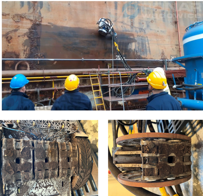
Figure 12: Adhesion modules on robot: robot working on ship, modules next to main wheels, module on secondary wheel
