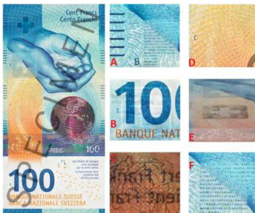
Figure 4. Selected security features of the Swiss franc based on the example of the denomination of CHF 100.
