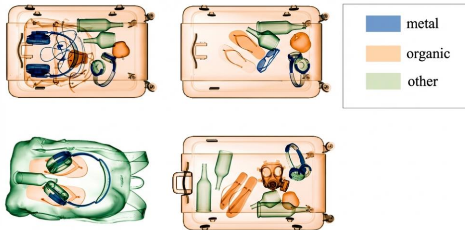
Fig 6. Output of the digital twin: simulated X-ray visualizations of baggage for comparison with real scanner images.
