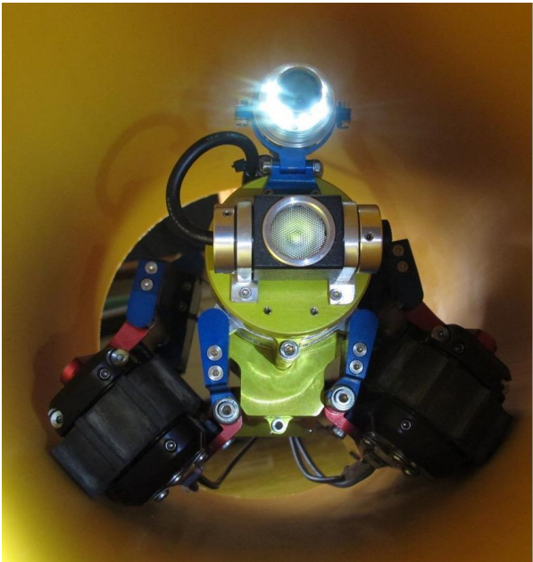
Fig. 2. Compact pipe inspection platform with articulated wheel modules arranged around the central body.
