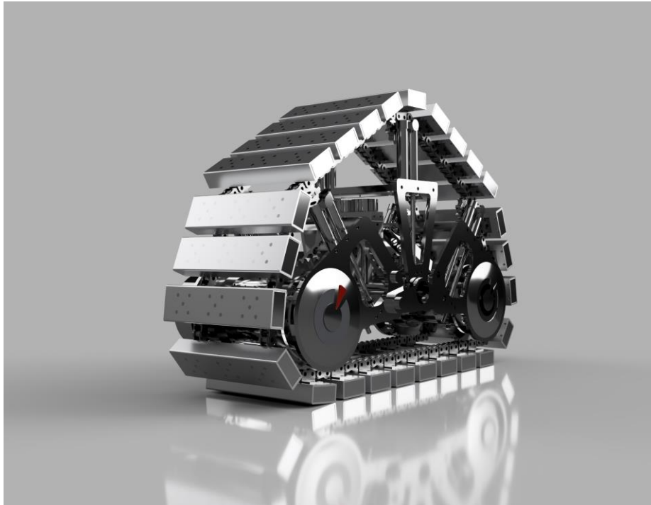
Fig. 5. CAD model of a magnetic track module showing the drive assembly, frame, and contact elements.
