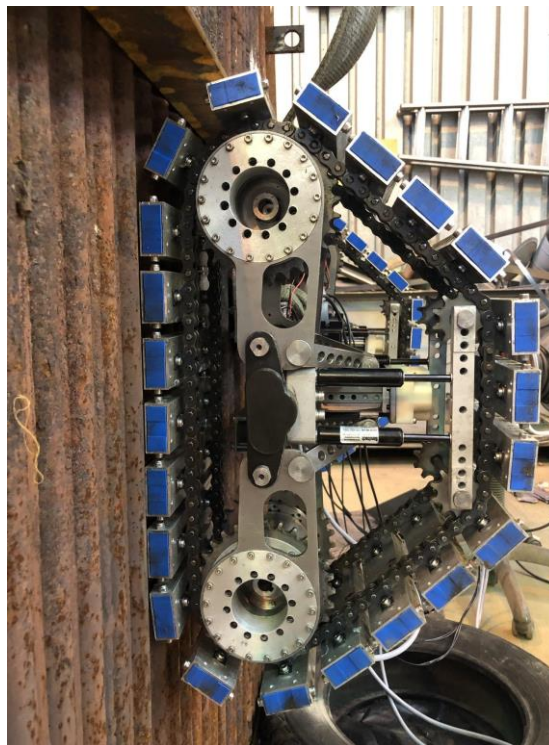
Fig. 4. Detail of a magnetic track module showing the distribution of magnetic elements along the track.
