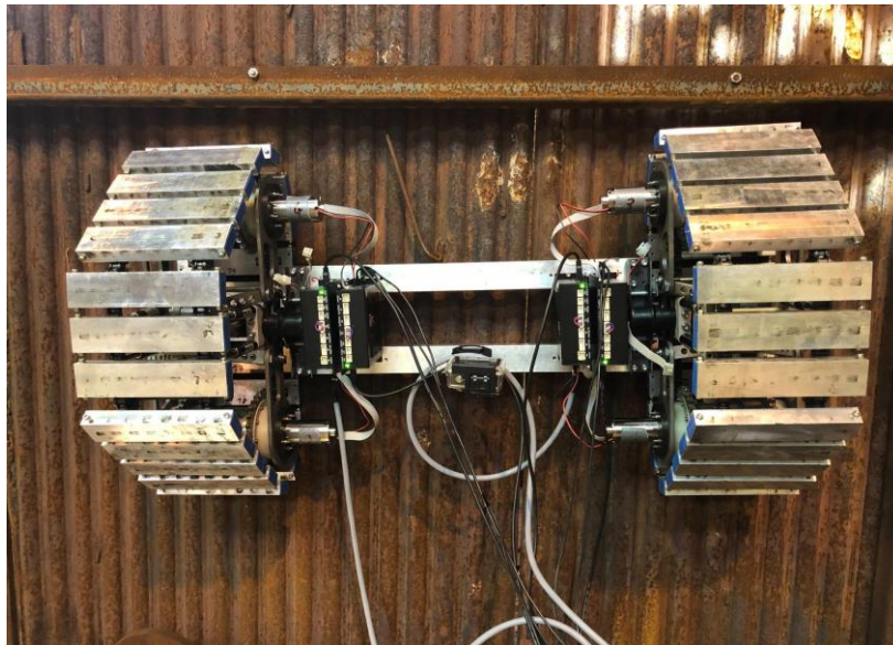
Fig. 3. Magnetic tracked platform operating on a vertical steel surface.
