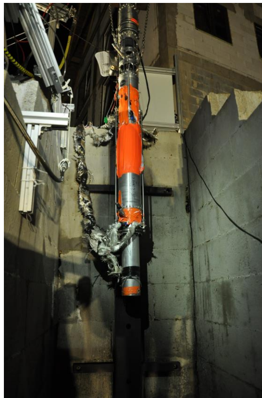
Fig 2. PWr in Space test stand right after the engine static hot-fire test
