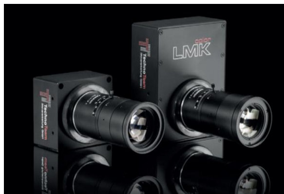
Figure 7. Photometric head with matrix image recorder used in the study
