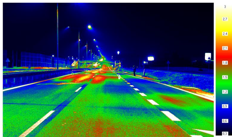
Figure 1. Example of road luminance measurement with a luminance matrix meter [Chrzanowicz et al. 2014].
