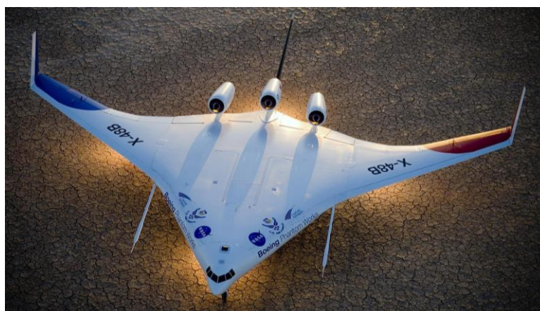
Figure 1. Advanced aircraft geometry concept – blended-wing body
