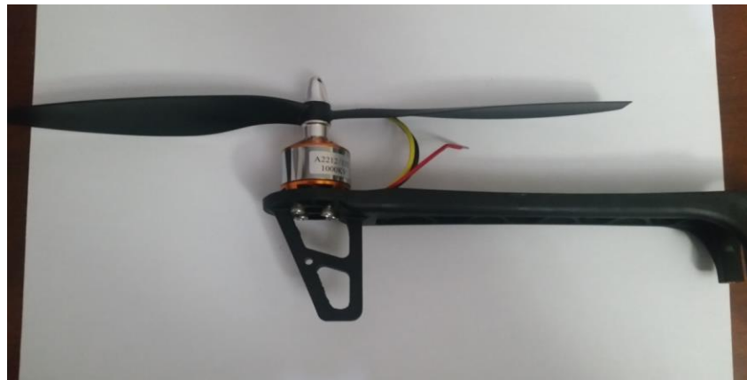
Fig. 7. Motor and propeller assembled on the arm
