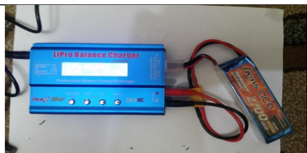
Fig. 6. Charging the battery using the BALANCE function
