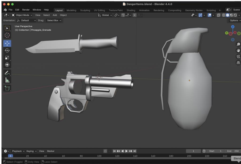
Figure 2. Blender-rendered views of the 3D dangerous item models used for the X-ray simulation.
