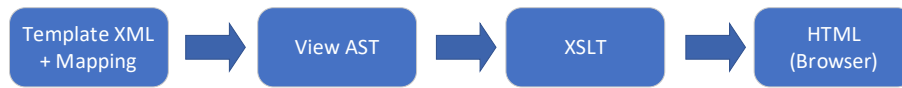
Fig. 1 Conceptual pipeline from template XML and mapping declarations to HTML via View AST and XSLT
