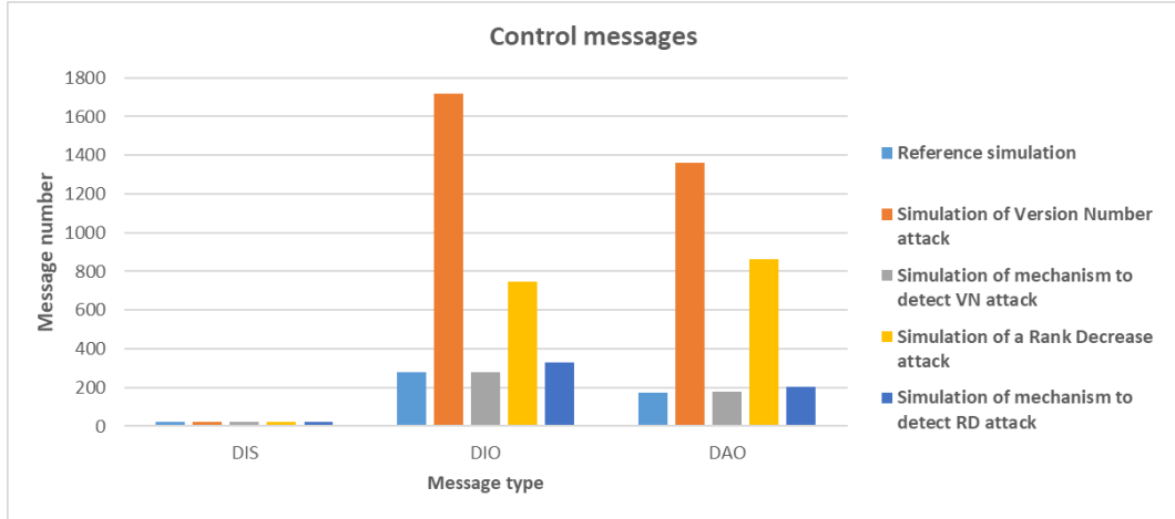
Fig 7. Number of control messages sent during testing of Version Number and Rank Decrease attack detection mechanism (Source (Own))
