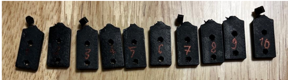
Figure 16 - Mixed materials, Alternative Method. Average highest strain torque:18.28Nm
