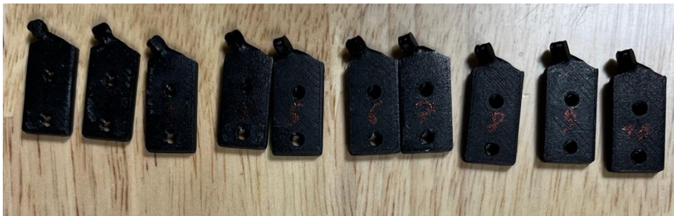
Figure 12 – PA12, Alternative Method. Average highest strain torque:14.04Nm
