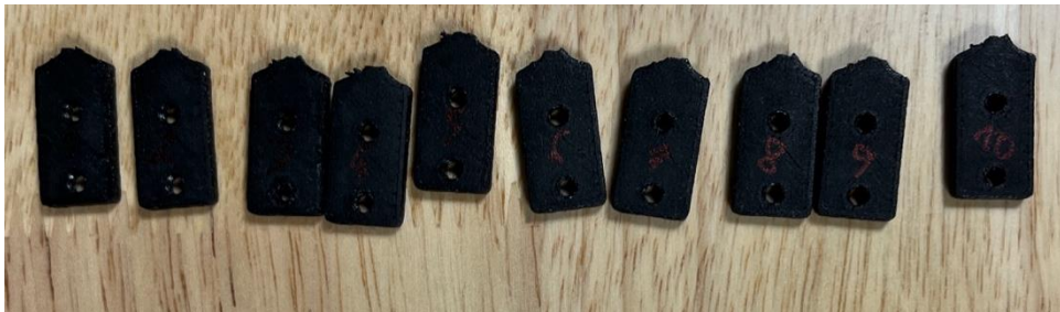
Figure 13 – PA12CF15, Standard Method. Average highest strain torque:18.96Nm
