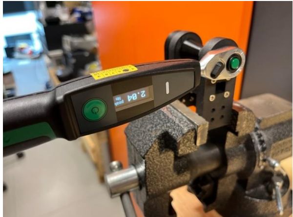
Figure 4 - Torque wrench in a test jig
