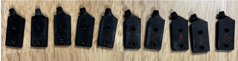
Figure 11 – PA12, Standard Method. Average highest strain torque:13.19Nm
