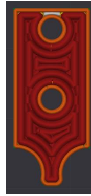
Figure 7 - Alternative method, single material, odd number layer profile
