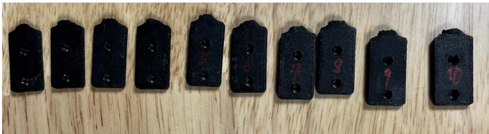
Figure 14 – PA12CF15, Alternative Method. Average highest strain torque:22.1Nm
