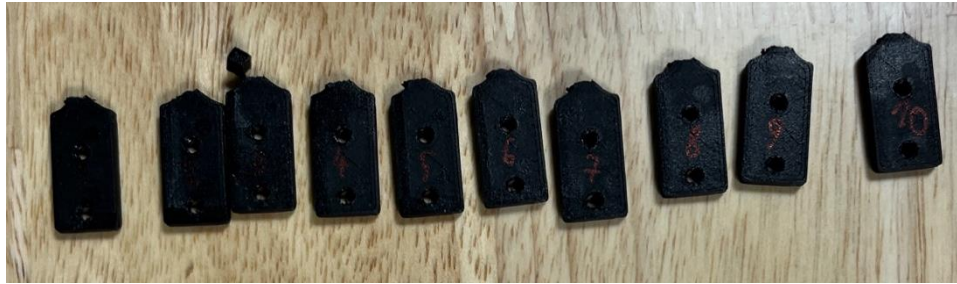
Figure 15 - Mixed materials, Standard Method. Average highest strain torque:18.8Nm
