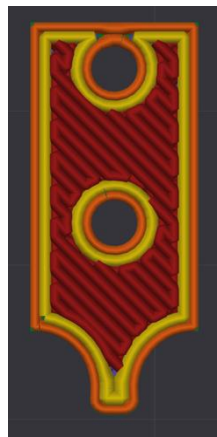
Figure 5 - Standard Method single material layer profile
