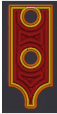
Figure 6 - Alternative method, single material, even number layer profile
